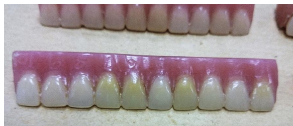
Figure 1: Ten teeth processed in a block of denture base material
